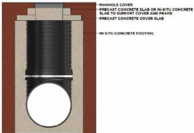
Figure 30: Illustration of access turret completely encased in concrete.
